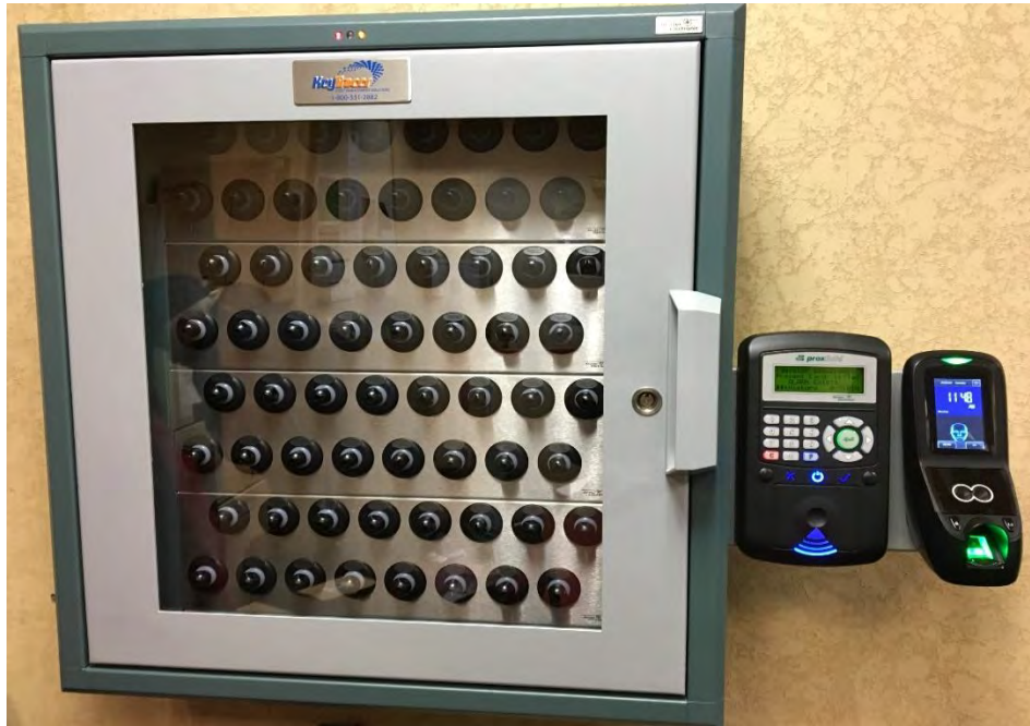
Daisy-chained KTA-4 Module Cabinet with KTA Terminal and Biometric Facial
